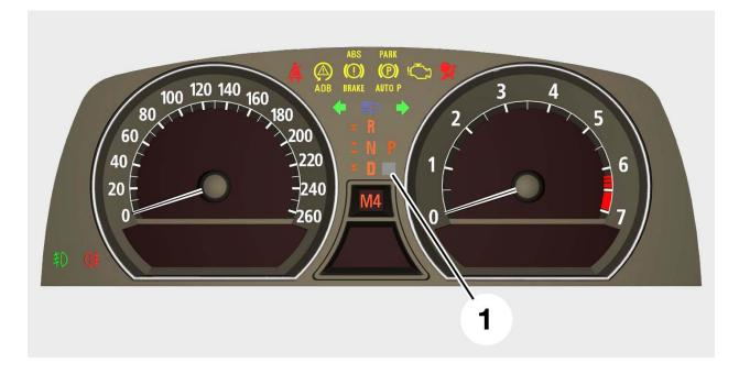
The brightness signal is calculated in the instrument cluster from the values of the phototransistor (1) and the dimmer wheel. This brightness signal is also made available via the K-CAN System to other control units in the vehicle. The instrument cluster is thus used as the "dimming master".
